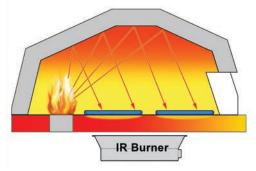
The Wood Stone IR burner heats from below-but only when high production requires the assist
